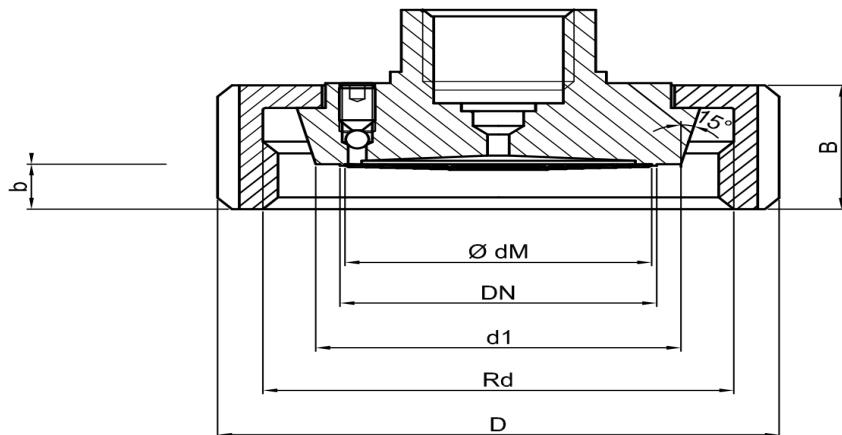
**Conical nut connections PN 40 bar**
